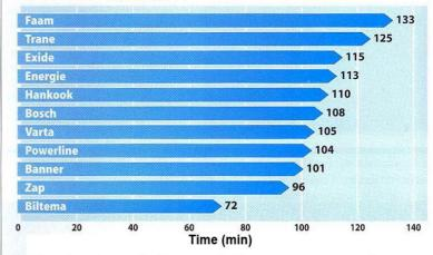
▶ IF a strap charger is disconnected for any reason, a good reserve capacity is required. It tells how long the power will get out of a battery until the end of charge.
