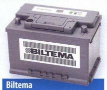
Model: 80-2752 75Ah Cold start current: 720 A (EN) Plates per cell: 19 pcs Maintenance free: yes Carrying handles: yes Display for state of charge: yes Dimensions (LxWxH): 277 x 174 x 175 mm
